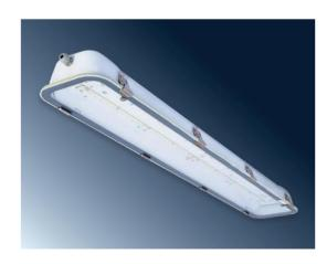
Suspended Industry LED Luminaire is intended to provide illumination in the production areas and in places requiring higher protection level. The fixture is made from steel frame painted in RAL 9003 color covered by tempered glass. The panel is based on LED modules with superb performance characteristics, long life span and economic operation.
